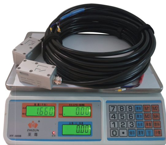
Transducer weight TT03: 1.66kg
