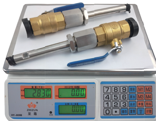
Transducer weight TT05:2.83kg
