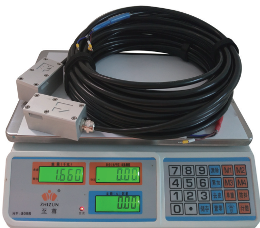
Transducer weight TT02H: 1.66kg
